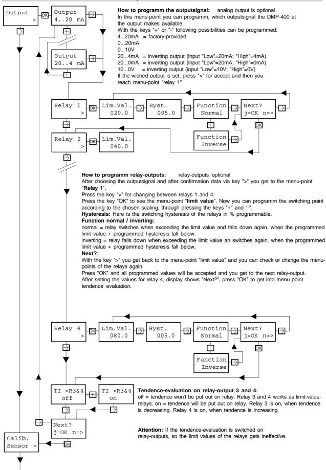
for Hydrocont P and analoge signals with LCD-display and 4 relayoutputs **operation instructions**TA 11.99 page 7 of 13
