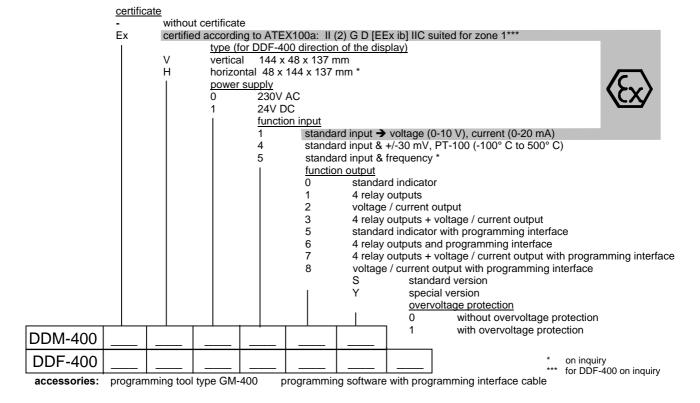
for 0..20 mA, 4..20 mA, 0..10 V, PT-100 or mV-differential signals with sensor feeding and 4 limit values
