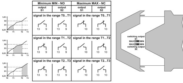
The configuration of the safety function per switching output is carried out by jumper, inside the device.
