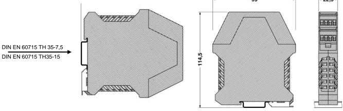
The device must be installed protected against dust and humidity, e.g. in control stations or in a suitable protection housing with a minimum protection classification IP55 acc. to DIN EN 60529.
